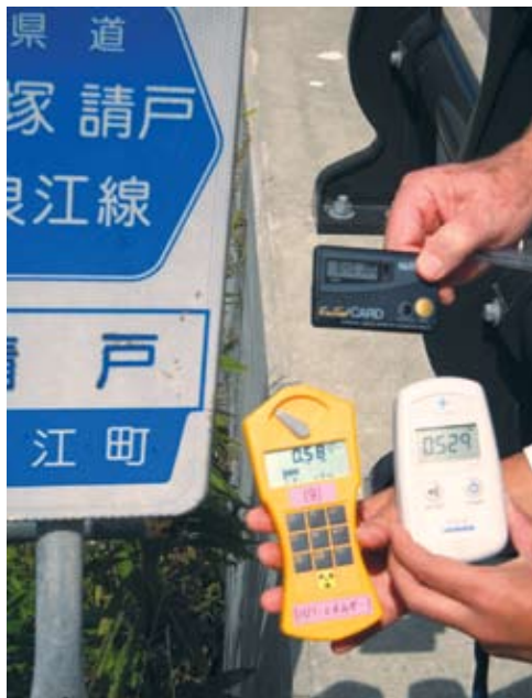
Three dosimeter readings at the coastal road bridge, showing 0.58, 0.40, and 0.529 millisieverts/hour.
