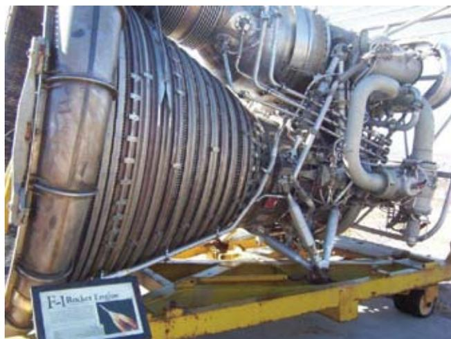
*The remains of a V2 rocket on display at the Museum (left) and an F1 rocket engine.*
