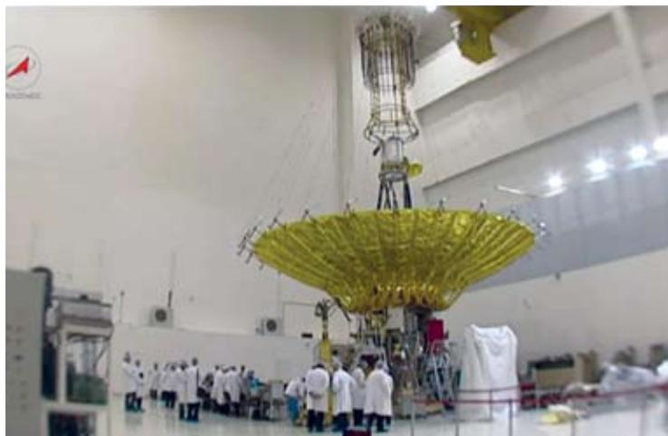
*Videograb of Spektre R being readied for deployment into space on the Zenit 3F rocket.*
