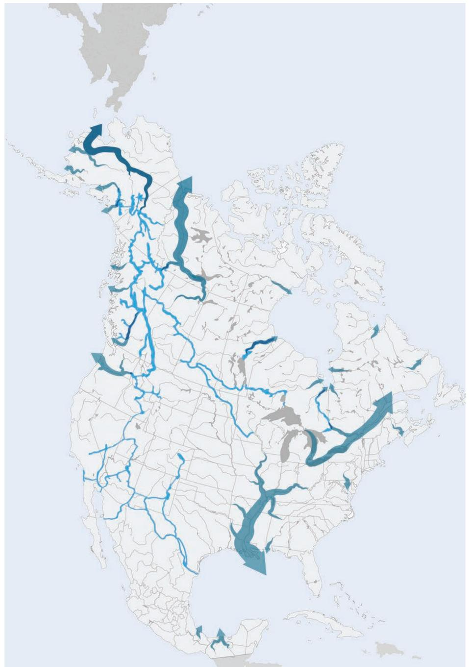
*The North American Water and Power Alliance, NAWAPA, would save massive amounts of freshwater from otherwise wastefully running off into the northern Pacific and Arctic oceans, by directing it down through a series of natural trenches, rivers, tunnels, canals, and reservoirs, into the western United States and northern Mexico.*
