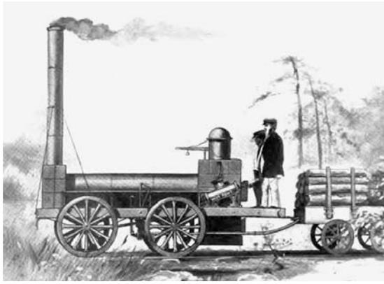
The "West Point" was the third steam locomotive built in the United States, and the first featuring a horizontal locomotive-style boiler. Its name is appropriate, because the West Point graduates who entered the Corps of Engineers were involved in surveying, designing, or supervising the construction of most of America's early railroads.
