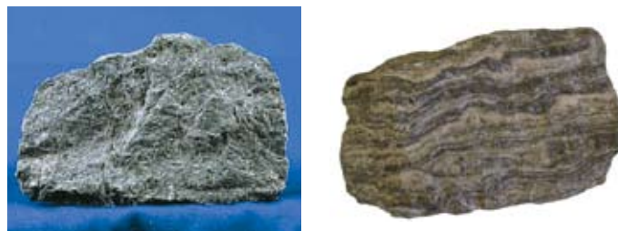
The conventional, statistically based theory holds that drilling 3 to 6 kilometers down, there would be a transition into basaltic basement rock (left). But the Kola borehole never reached basalt; they found gneiss (right), which was so hot that it destroyed drill bits.
