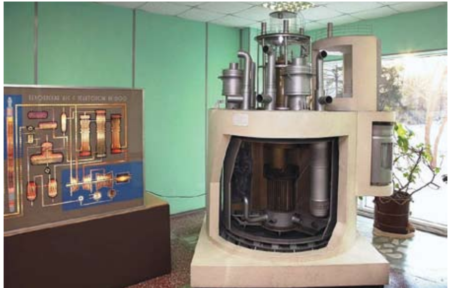
A cutaway model of Russia's BN-600 fast reactor.
