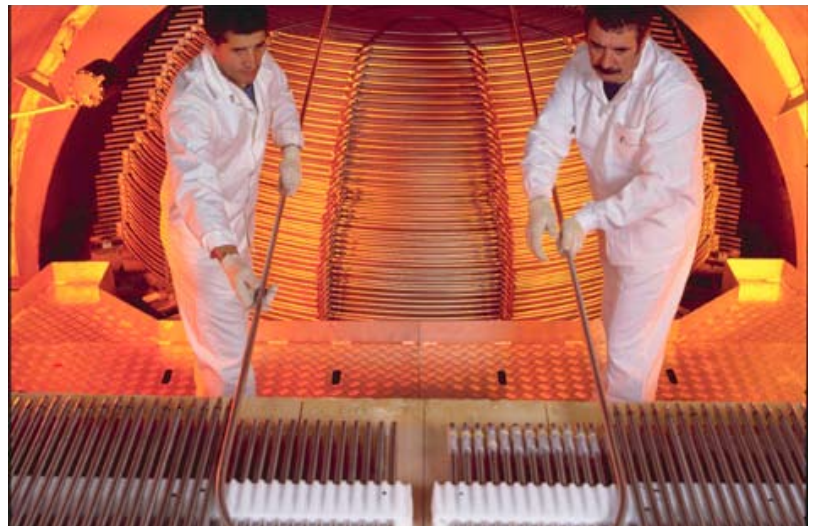
Tube for a nuclear steam generator being manufactured at the Chalon Saint Marcel plant in France. Production capacity for smaller nuclear components must be geared up worldwide.
