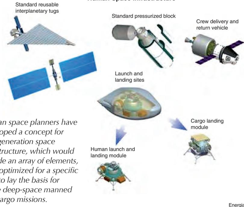
Russian space planners have developed a concept for next-generation space infrastructure, which would include an array of elements, each optimized for a specific task, to lay the basis for future deep-space manned and cargo missions.
