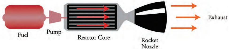
*Comparison between chemical and nuclear thermal rocket operation. In a chemical rocket (top), the fuel is combined with an oxidizer, ignited, and the explosive reaction directed out the rocket nozzle. In a nuclear thermal rocket, liquid hydrogen is flowed through the reactor core and heated to extreme temperatures, which forces it to evaporate and expand, and it is then directed out the rocket nozzle.*
