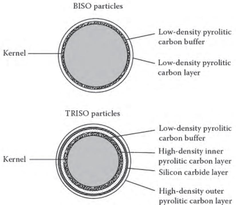
*Bi-isotropic ("biso") and tri-isotropic ("triso") nuclear fuel pellets. Both pellets contain a kernel of uranium fuel, coated by several layers of material.*
