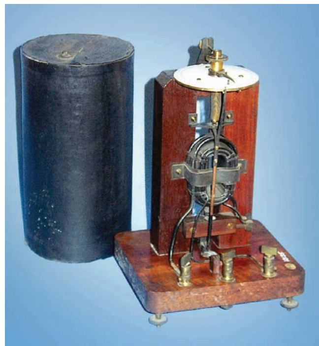
A later model of Weber's electro-dynamometer, which was built by Siemens Bros.
