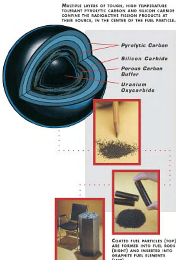
Figure 2 THE UNIQUE HTR FUEL IN A PRISMATIC CONFIGURATION (GT-MHR)
