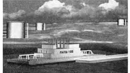
Top: An artist's drawing of the Russian design for the first commercial floating nuclear power plant. Below: The USS Sturgis , providing nuclear electricity in the 1960s.
