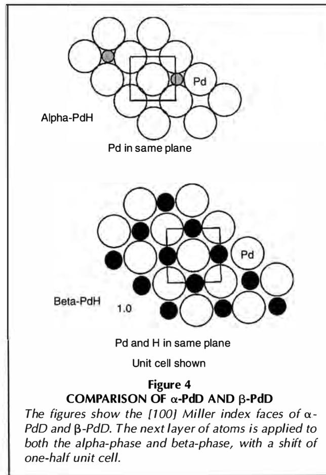
mined by comparing the expected lattice volume, based on the composition, to the measured volume.[114] In forming the  $\beta$ -phase, atoms of Pd shift to allow D atoms into equivalent positions, as shown in Figure 4. Hydrogen lies in the plane, forcing Pd atoms further apart, and occupying the so-called octahedral position. These positions can be filled or empty in a random manner up to a completely filled lattice at PdH<sub>1.0</sub>.
