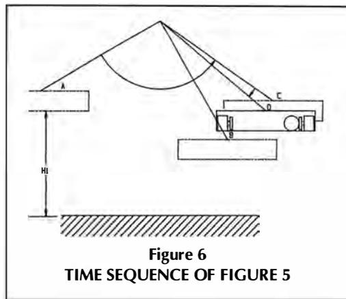
moving upward toward the right side zenith. At Point B, the left solenoid is fired, pushing the ball to the right (Figure 5). Point B has been chosen to be a position somewhere along the chamber's upward trajectory. Because of action/reaction, some of the rightward momentum of the pendulum is cancelled.
