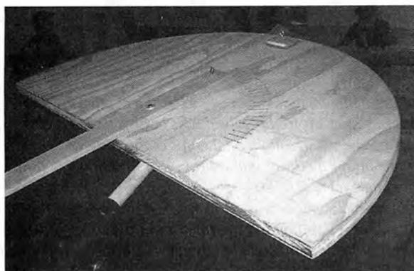
*Jermaine Hughes demonstrates the use of one piece of apparatus used for Mars measurement in Los Angeles over the past summer. The close-up helps to show some of the technique and technology used. The instrument is essentially an oversized protractor, which in this instance was mounted onto a microphone stand with a universal joint, using a wooden dowel which made it easy to align and adjust the whole contraption to the*
