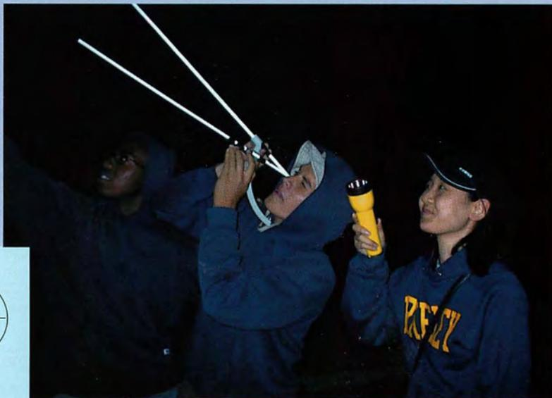
*From left: Summer Shields, Oyang Teng, and Lee Miok demonstrate how to measure the angular distance of Mars from nearby stars, using a device adapted from a Lenart Sphere protractor. The flashlight illuminates the tips of the dowels inserted into the spherical protractor.*
