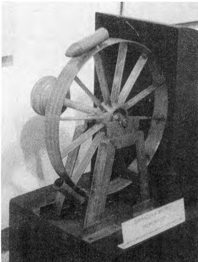
*Pedro Paulet's Girándula consisted of rockets attached to the outside of a wheel, to be fed fuel through tubes in the spokes. Ignition was provided by spark plugs, similar to those used in automobiles. The rocket exhaust caused the wheel to rotate.*
