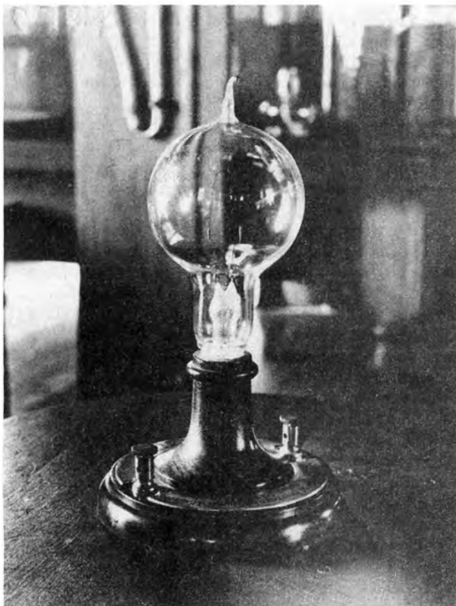
"We still do not know what electric currents really are." Here, a replica of the first successful incandescent lamp, invented by Thomas Edison in 1879.
