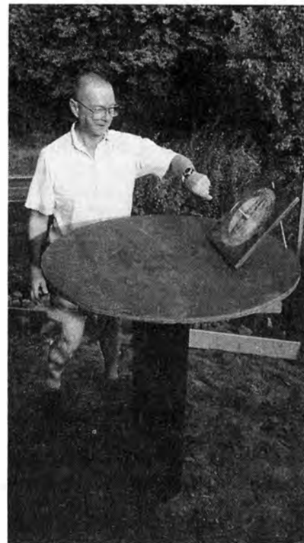
The author, using an equatorial sundial to establish a north-south line.
