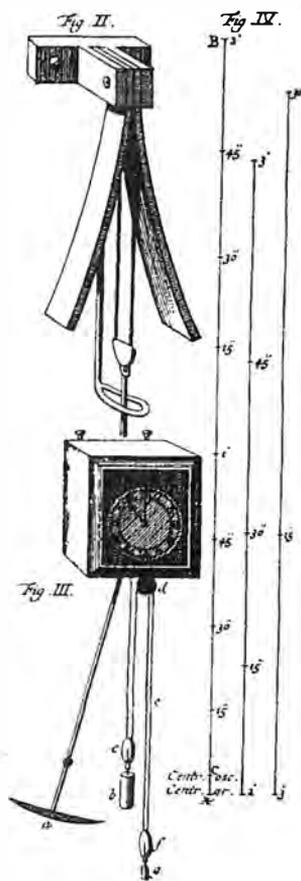
The pendulum clock (ca. 1658) designed by Leibniz's collaborator Christiaan Huygens. The pendulum is suspended by a flexible band which wraps around a segment of a cycloid curve as it swings. Because the cycloid curve is its own evolute, and is isochronic, the clock keeps equal time regardless of the amplitude of swing.
