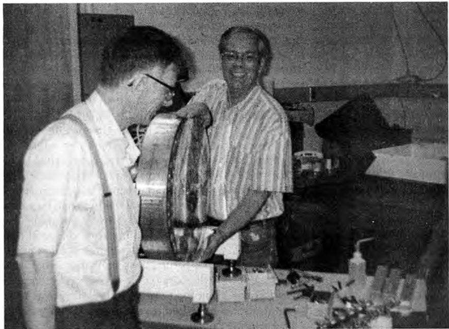
The Steward Observatory Mirror Laboratory, with the encouragement of NASA administrator Dan Goldin, has made a prototype of a 6.5-meter mirror that will be only 2 millimeters thick, as a candidate for the Next Generation Space Telescope. Here Angel, holding the $50,000 prototype in his gentle hands, shows the author how the mirror rests on an array of 36 actuators.
