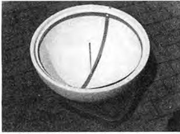
Hemispherical sundial, built for replication of Eratosthenes' experiment.
