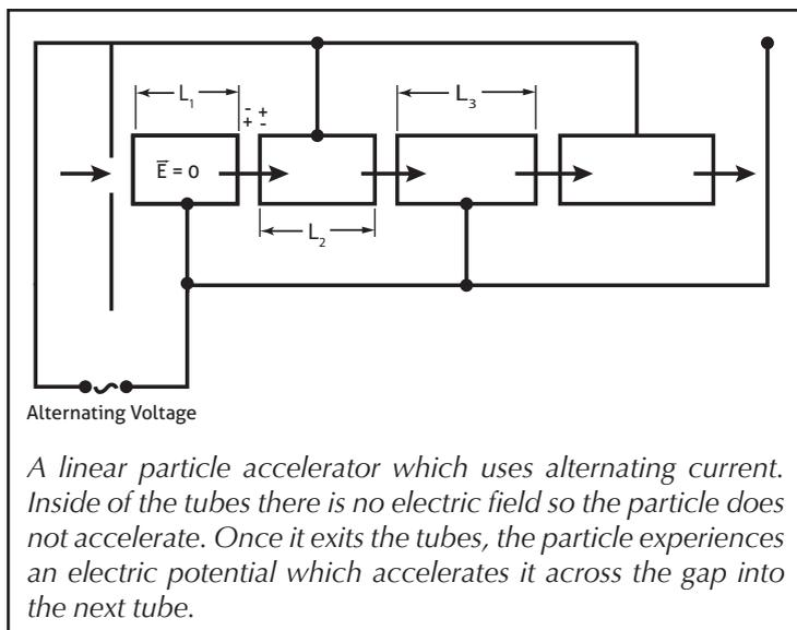
the proton is charged, it can be influenced and accelerated by a voltage difference. By placing several voltage differences in succession, they were able to accelerate a particle to 800,000eV.<sup>6</sup> At this potential, a proton would be accelerated to about 12,000 km/s.
