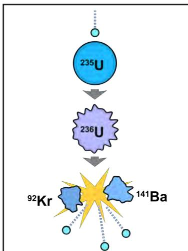
When uranium-235 is bombarded by a neutron, it fissions, or splits apart. Besides its fission fragments, it also releases neutrons, stimulating other uranium atoms to fission, etc., resulting eventually in a self-sustained chain reaction, and a continuous energy source, until so much of fuel has been converted that the reaction is no longer self-sustaining.
