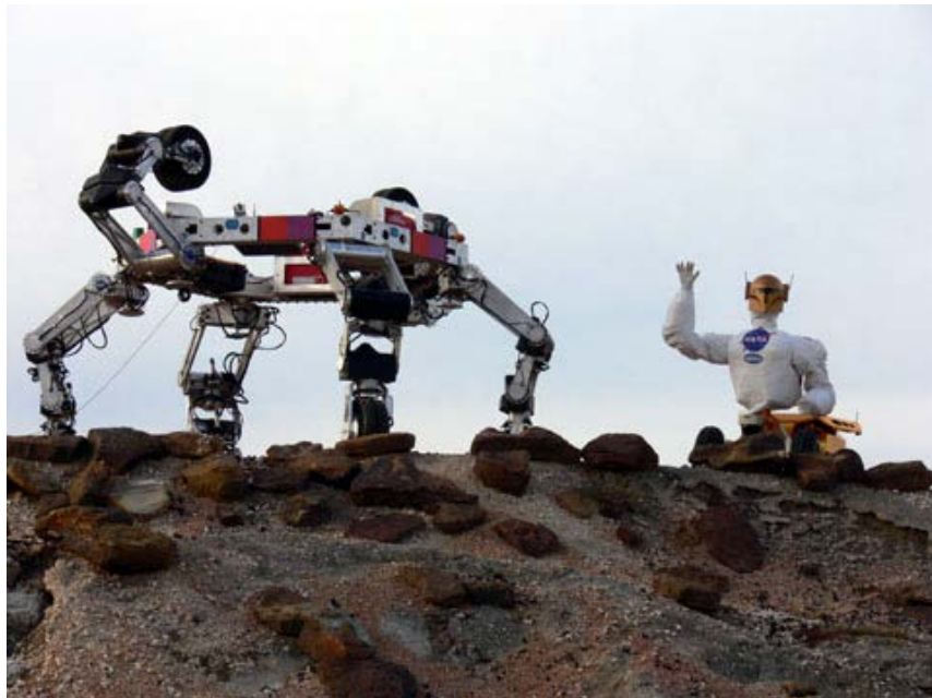
The All-Terrain Hex-Limbed Extra-Terrestrial Explorer (ATHLETE) vehicle.
