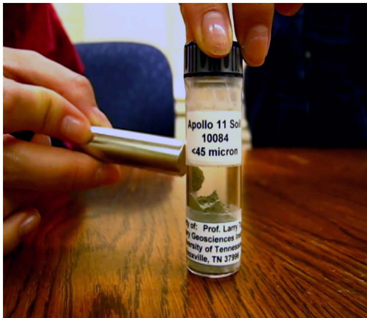
A fine-grained lunar soil sample from Apollo 11 is easily attracted by a hand magnet.
