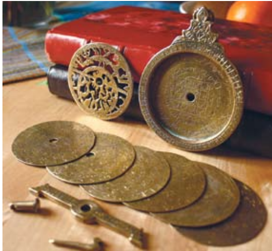
Figure 5 AN ASTROLABE DISASSEMBLED An 18th Century astrolabe from North Africa, showing its various parts. The axle and linchpin device are in the foreground.
